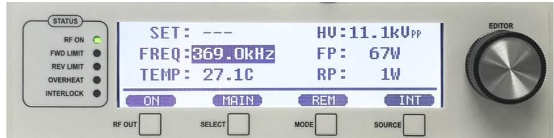
**EDITOR knob** offers two movements. Left and right rotations, to decrease and increase the value in the cursor field. By pushing that knob, cursor changes the adjusting field, for example from SET: to FREQ:
