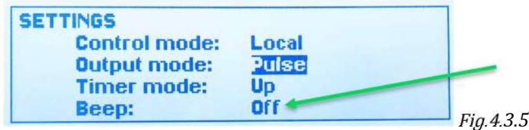
Turn rotary encoder or use arrow buttons ▲ or ▼ to select *Beeper* field; press **ENTER** button or rotary knob to edit. Press **ENTER** button or rotary knob again to confirm the settings.
